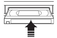
The TV/VCR automatically turns on. If the erase-protection tab has been removed from the cassette, playback automatically begins (see "Erase Protection" on Page 26) and **PLAY** appears on the TV screen for about 4 seconds.
